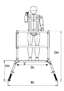
▶ THREE optional platform levels between 550mm and 700mm will suit most low-level requirements.
