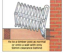
Sovereign Stairway is suitable for use in a variety of applications. It can be bolted to a joist above a trapdoor as normal, or it can be bolted to a wall where no trapdoor exists. When bolted to a wall an extra 50mm of packing must be fitted behind the backboard to ensure it can rotate correctly into its stored position.
